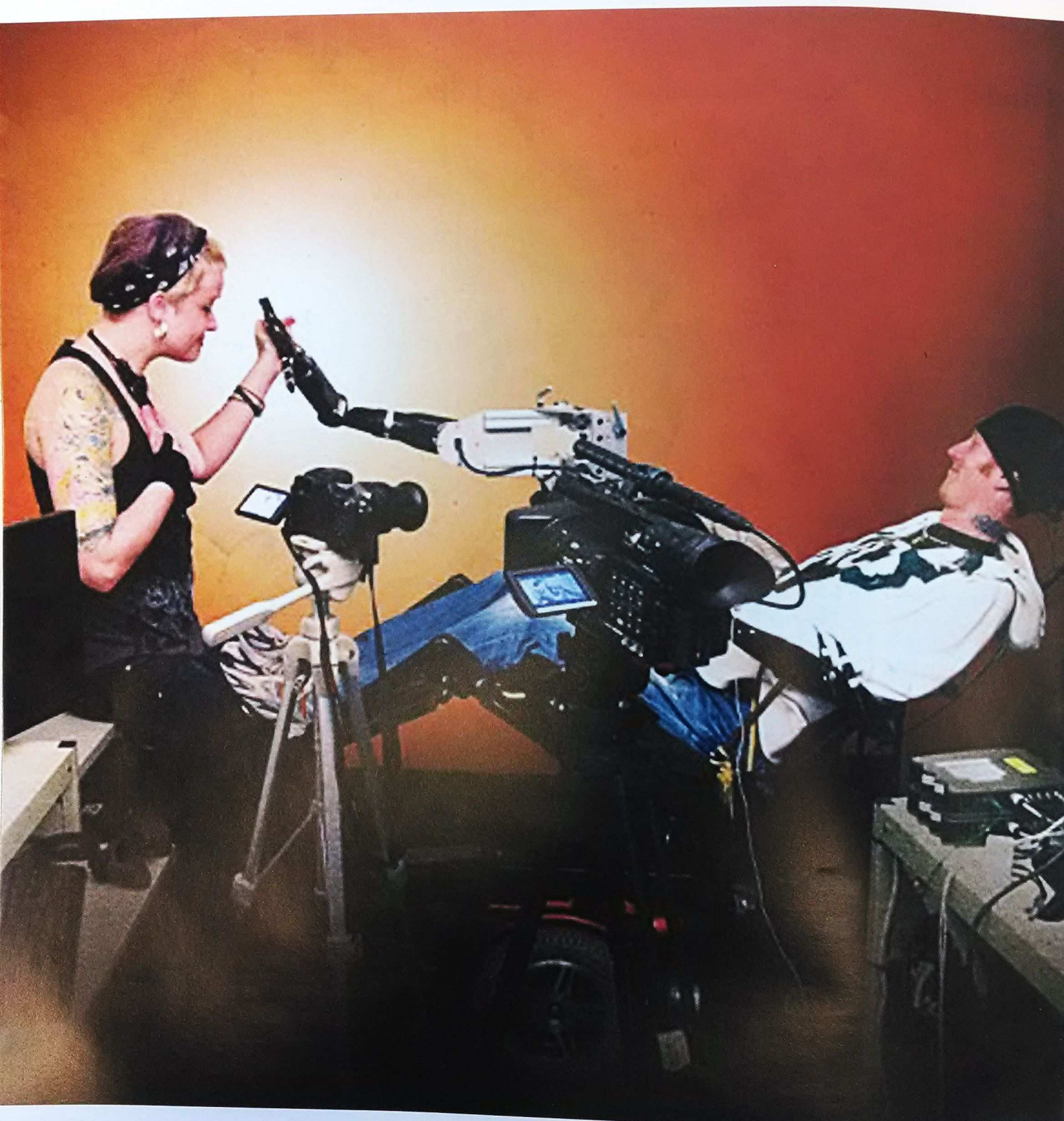
For the first time in seven years, Tim Hemmes touches his girlfriend's hand; to do so, Hemmes uses a robotic arm he controls with his thoughts.
