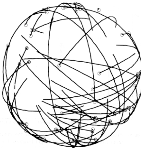
Fig. 4: Changes in preferred direction between arm control and final brain control. Each line is the projection onto a unit sphere of the change in preferred direction of an individual neuron between the arm-control task (blank end of line) and the adapted brain-control parameters (indicated by circles). Open circles are for neurons contralateral to the arm used in the arm control task, and filled circles are for ipsilateral neurons. All neurons shown had significant directional tuning in both the arm-control and the brain-control tasks.
